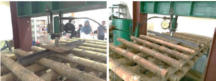
Fig. 7. Loading tests on bamboo mattress.
